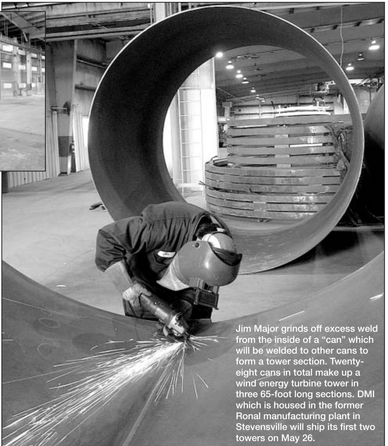
Jim Major grinds off excess weld from the inside of a “can” which will be welded to other cans to form a tower section. Twenty-eight cans in total make up a wind energy turbine tower in three 65-foot long sections. DMI which is housed in the former Ronal manufacturing plant in Stevensville will ship its first two towers on May 26.
